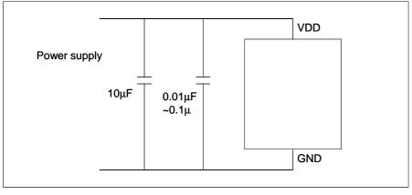
Please connect a bypass capacitor immediately near the power supply terminal. A capacitor should connect 0.01 uF ~ 0.1 uF and 10 uF to the arrangement in a row.
