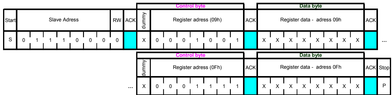
Figure 15: I 2 C multiple write protocol
