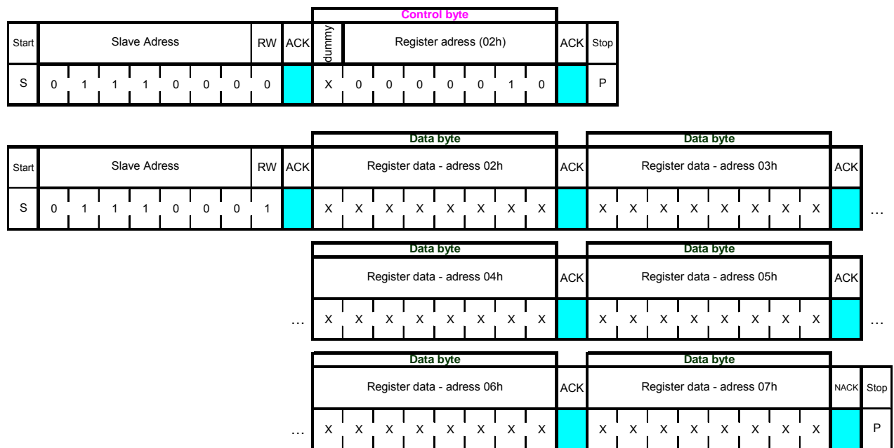
Figure 16: I 2 C multiple read protocol. Address register is first written to BMA150, the RW=0 (lowest acceleration data located at address 02h). I 2 C transfer is stopped and restarted with RW=1, address is automatically incremented and the 6 bytes can be sequentially read out.
